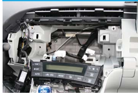
Step 2. Locate all the factory wires
