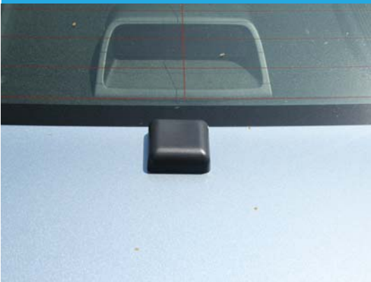
Step 1. Mount GPS and Satellite radio antenna
