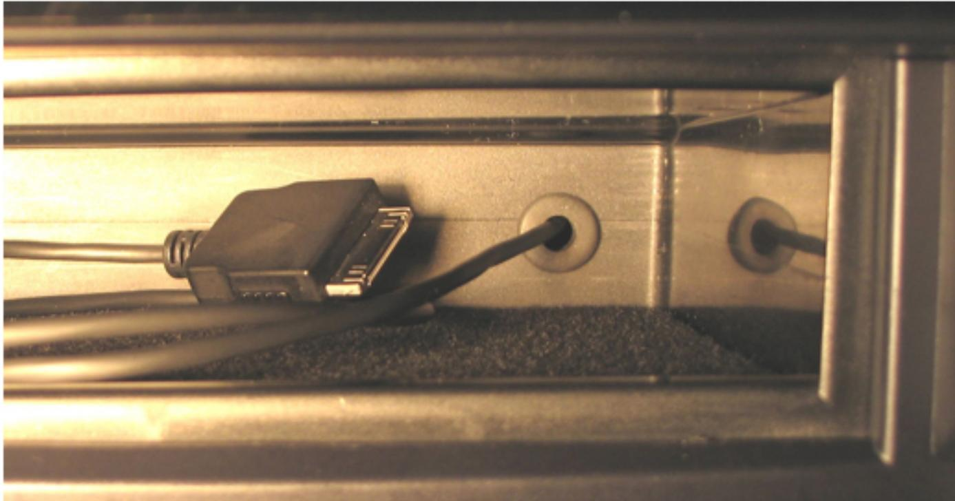
Feed round plug of iPod connection cable through hole in back of CD storage box and push grommet into place. It is helpful to have one finger behind box when pushing grommet into place.
