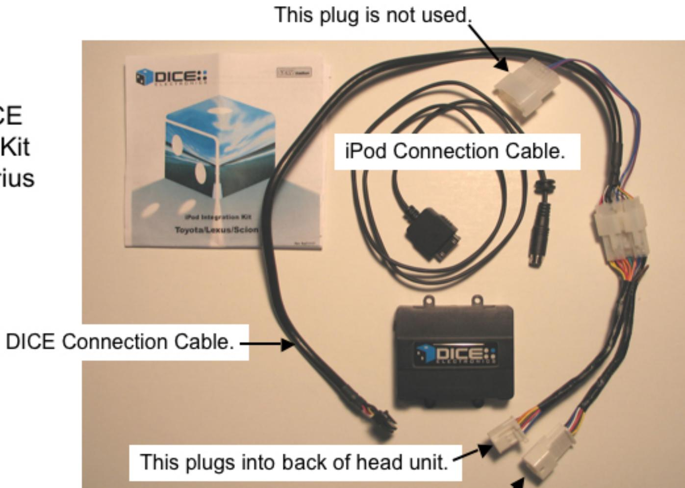
This is for Satellite Radio or External CD changer (not used normally).
