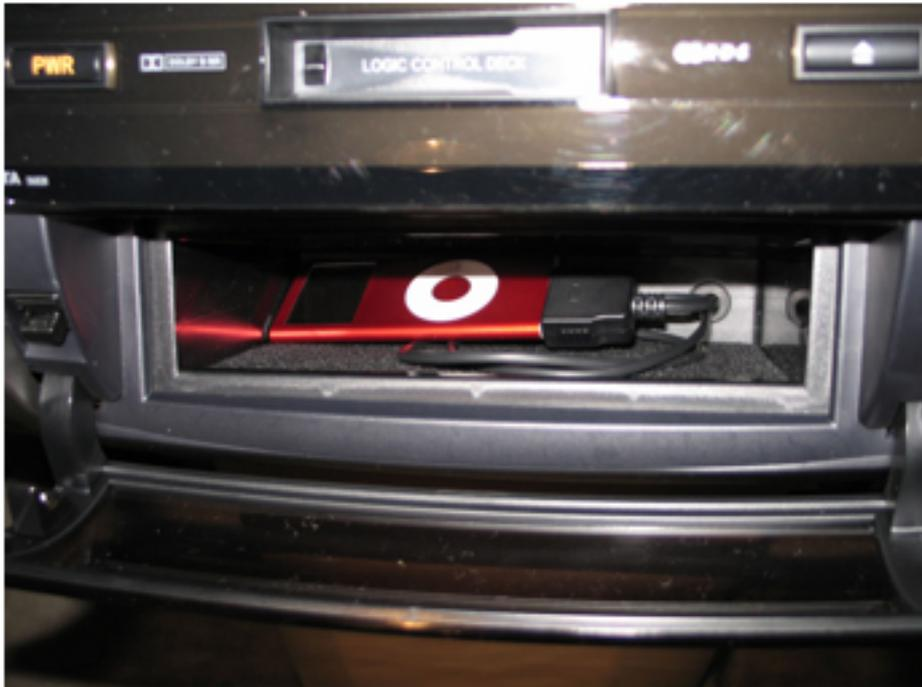
The CD storage box is a convenient location in your 2004-2007 Prius for your iPod when installing the DICE iPod Integration Kit.
