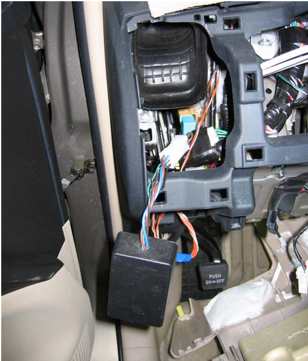
Here is a photo of the timer circuit installed in the plastic case. A 6 pin Molex connector was used to interface the circuit to the Prius dome light circuit.
