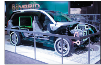
Figure 3– The Saturn Vue Green Line Hybrid vehicles use a Belt Alternator/ Starter type start/stop hybrid system.
