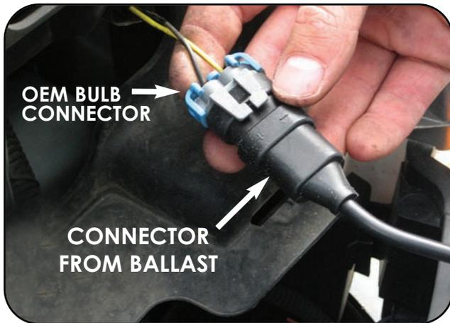
Insert the male 9006 connector (the connector that comes out of your OEM 9006 bulb) into the female 9006 connector coming out of the ballast. Mount ballast with the double sided tape provided to a clean flat surface in the engine bay.
