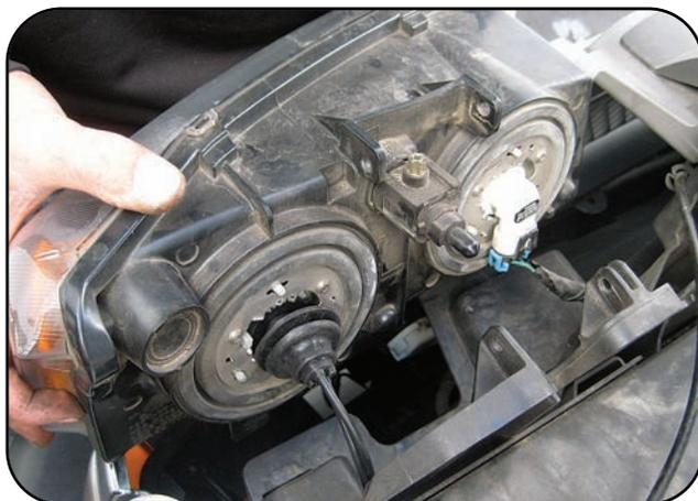
Slide the rubber grommet up to the bulb plug which keeps the bulb protected from the elements.
