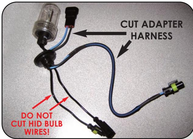
Adapter harnesses are not necessary for the 9006 HID kit installation. If desired you can cut and remove the adapter harnesses as pictured to left.
