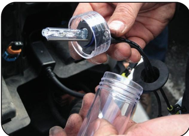
Remove the HID bulb from the protective plastic casing and screw cap. Do not touch the bulb with your bare hands. If you do, be sure to clean the bulb with rubbing alcohol prior to installation.
