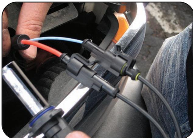
Connect corresponding AMP connectors from the ballast to bulb.
