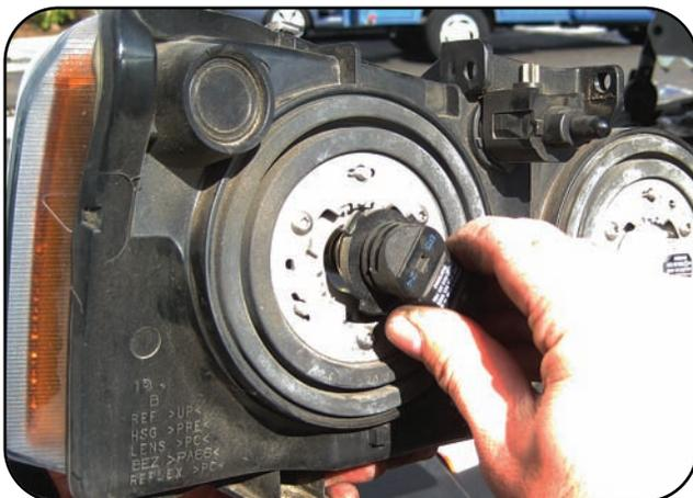
Twist OEM bulb counter clockwise to unlock the bulb from headlight housing. Once the bulb is unlocked remove gently from housing. **3**
