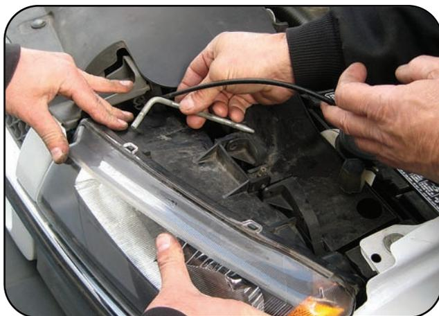
Reinstall headlight assembly if removal was required.
