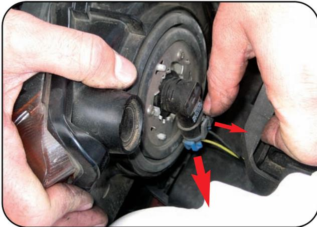
Open hood. Looking down from above into the engine bay and locate the low beam bulb. Remove retaining clip on 9006 low beam by simultaneously unclipping and pulling the connector away from the bulb. **1**
