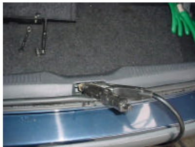
Earth connection on striker plate
