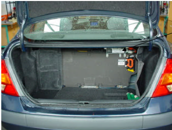
Rear Luggage Compartment Rear Panel Removed - Showing 12 volt to 300 volt inverter
