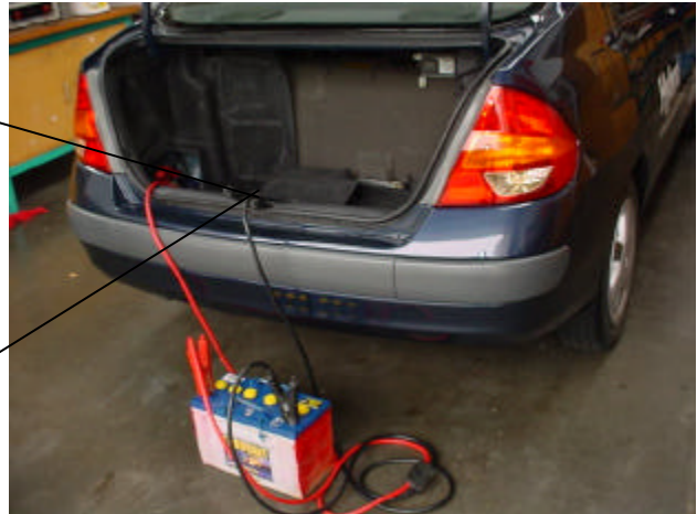
Photo showing large capacity battery connected to the 12 volt auxiliary battery positive terminal and striker plate for luggage compartment lid (boot lid).
