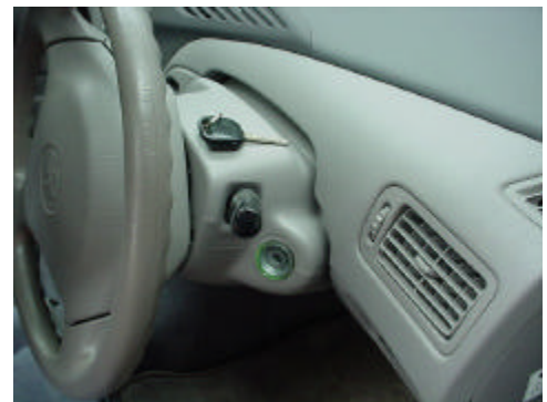
Photo showing ignition key removed from the ignition prior to “jump starting” the high voltage battery
