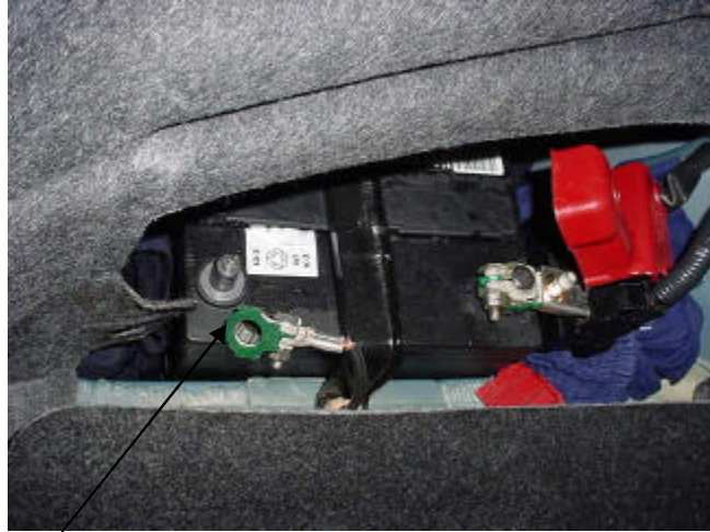
Photo showing negative terminal disconnected from 12 volt battery
