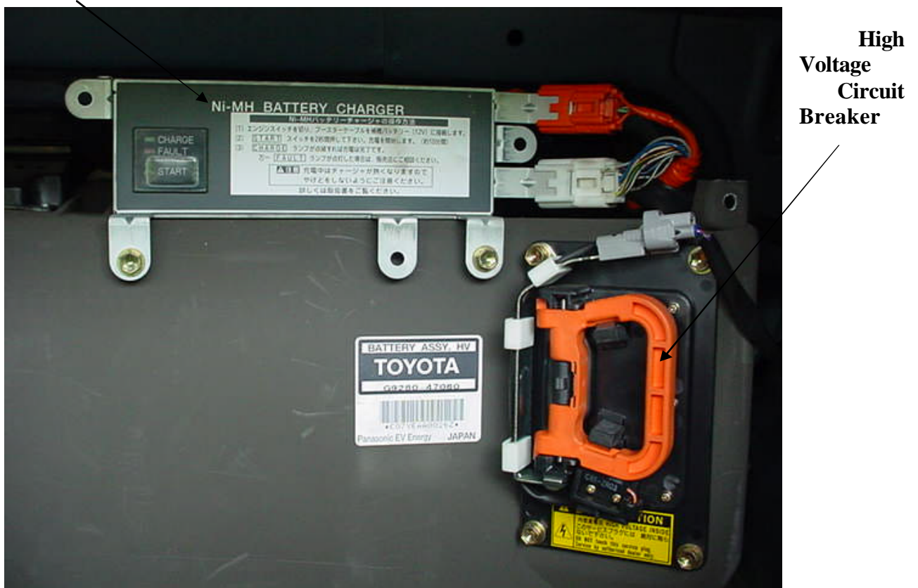
Close up view of Inverter and High Voltage Circuit Breaker located on hybrid battery pack
